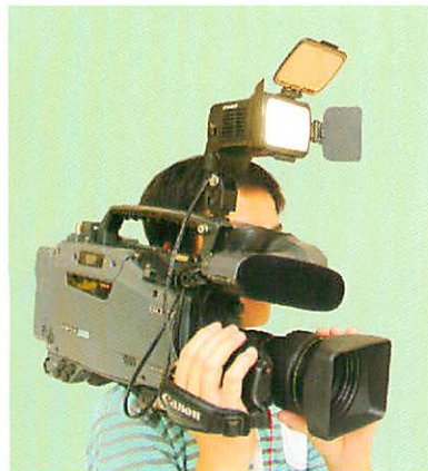
5: Hold the Video Camera on shoulder (share the battery pack with the Video Camera)
